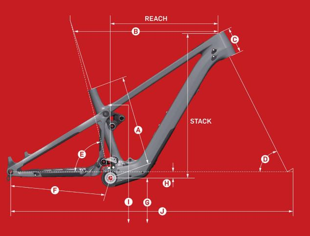
\* Effective seattube angles are calculated at an average saddle height for each size frame.
