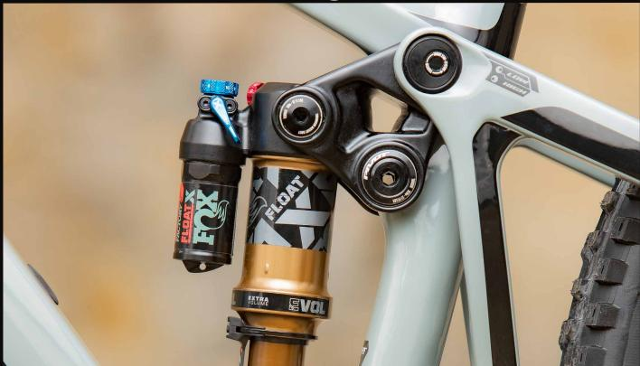
Allows a more compact frame design - stiffer, lighter, uses less material Increased shock rate progression Excellent water bottle clearance - fits large bottle sizes Full control over standover height
