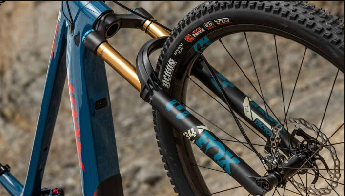
Fox Factory E-Tuned 34 29" 140mm on World Cup Builds Fox E-Tuned 36 29" 150mm on the Ride and Pro options Unmatched suspension performance and handling
